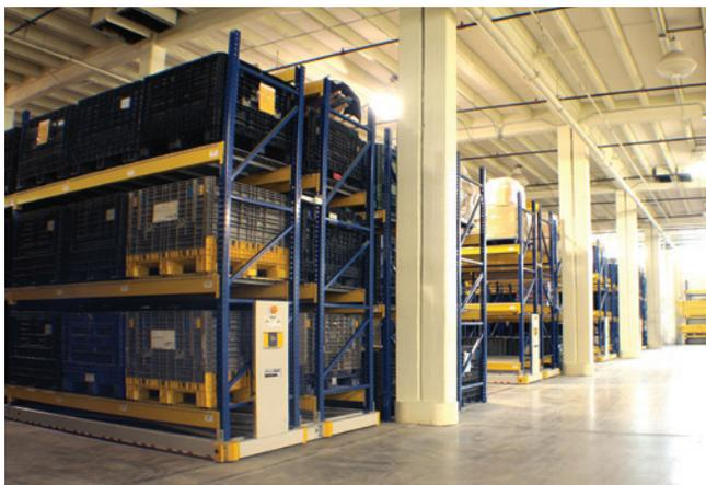
Spacesaver's **ActivRAC**® 16P System is ideal for heavy applications and features aisle activation via app, touchpad, Gesture Control™, and RF remote. Every system is custom designed to fit around columns or other structural constraints.
