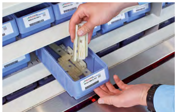
... and it is identified optically on the container or tray
