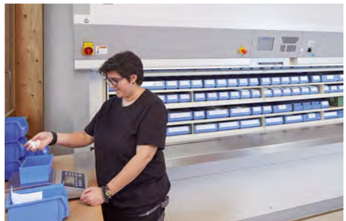
Loose parts are counted by weight on a scale near the storage system and then delivered to the assembly area
