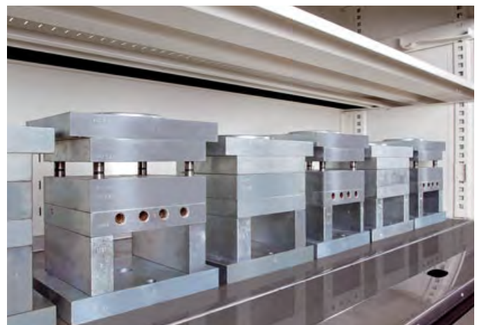
Tool storage in the Rotomat® industrial storage system
