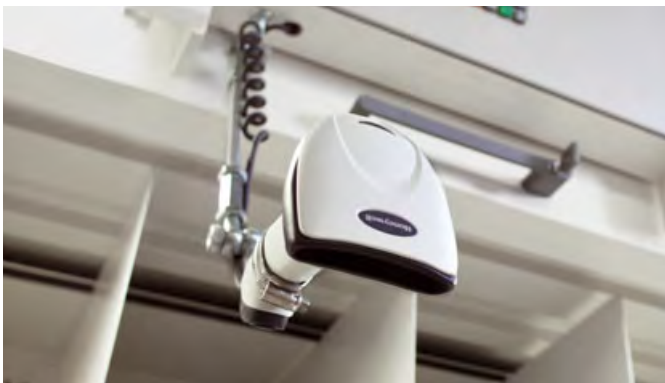
Rapid data entry for articles with the fixed-mount barcode scanner
