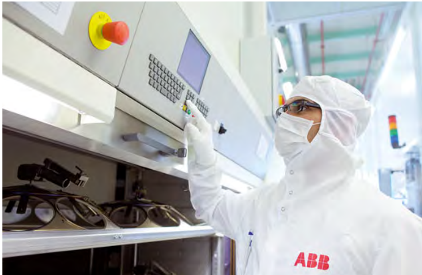
Storage of contamination-sensitive products up to clean-room class 5 according to DIN EN ISO 14644-1
