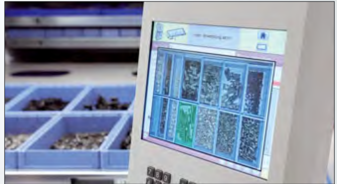
A container image is created after item retrieval and confirmation on the control unit
