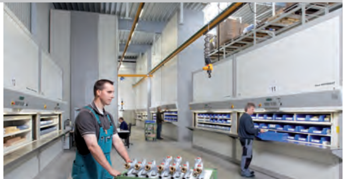
Buffer storage of parts and components needed in the production area
