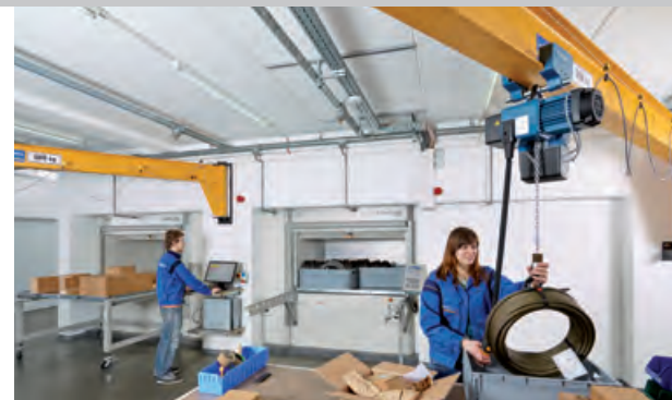
High throughput is achieved with two retrieval points that allow for simultaneous order picking
