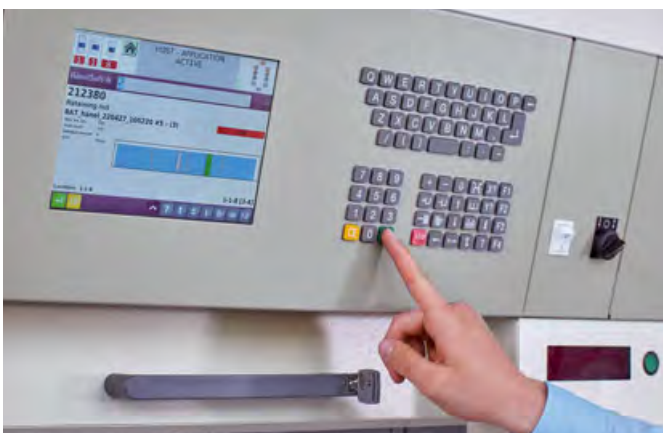
An image of the storage position is shown on the controller display...
