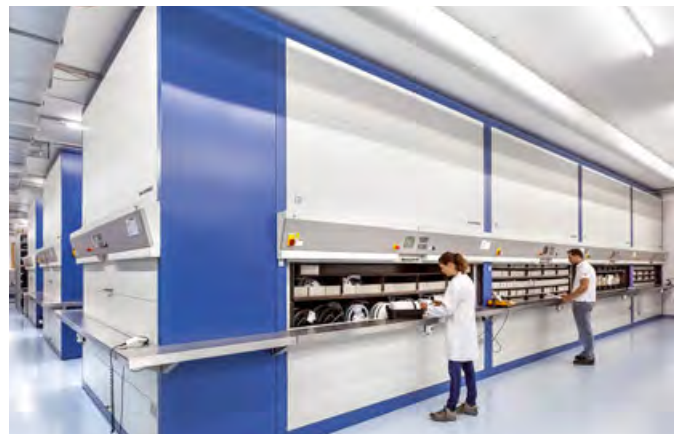
Diverse SMD components are neatly, securely and safely stored in the Hänel Rotomat® system
