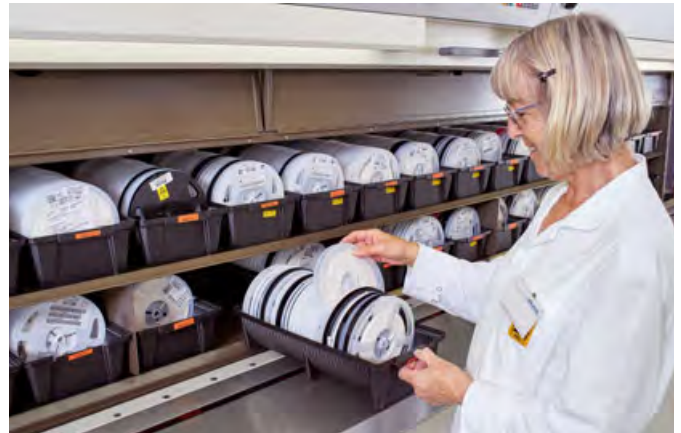
ESD buffer store for PC board assembly
