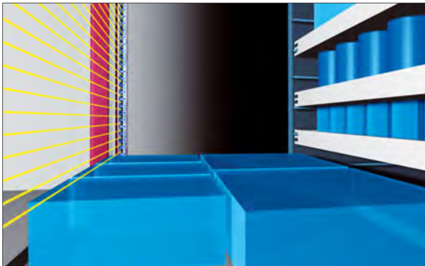
The items are measured in the access point by the height sensors
