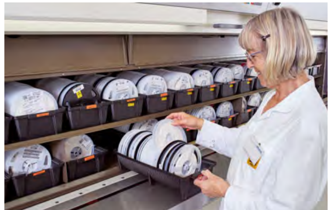
ESD buffer store for PC board assembly
