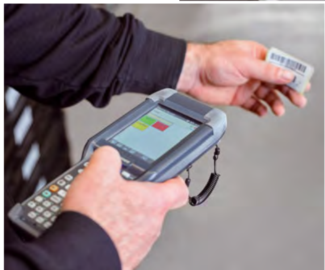
Articles are requested by entering a number on the controller or by using a barcode scanner
