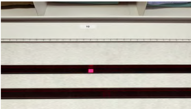
The double-row compartment indicator reliably shows the correct storage location
