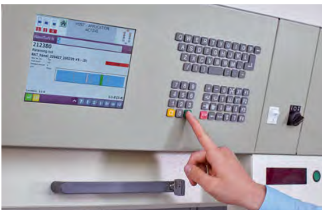
An image of the storage position is shown on the controller display...
