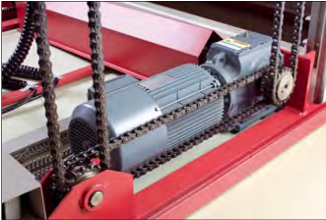
Highly efficient and powerful motors allow the extractor to achieve travel speeds of up to 2.30 m / 7.54 ft per sec
