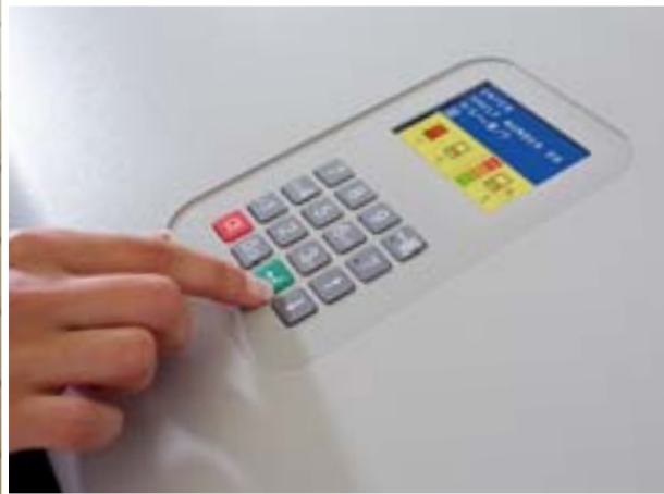
The Hänel MP ON controller with four-line information display and easy-to-follow operator prompts
