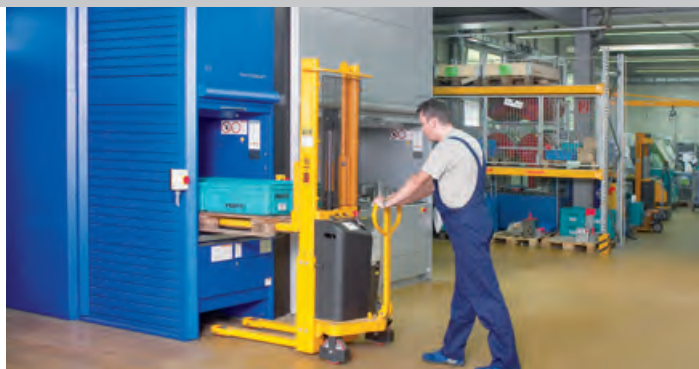
Integration in a modern building on two floor levels, with storage input supported by a Hänel Lean-Lift® pallet system on the ground floor
