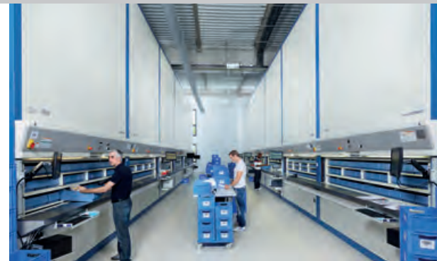
The Hänel Rotomat® storage carousel ensure that small parts are retrieved quickly and efficiently
