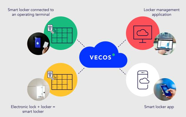
The hardware, usually in the form of an electronic lock, is connected to an operating terminal, which is then connected through the internet to a Software-as-a-Service (SaaS) platform. This software platform is the most critical component of a successful smart locker system, as this is where an
