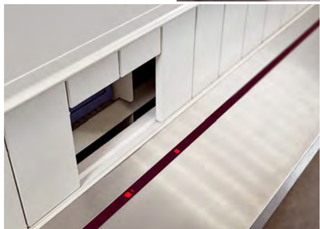
The compartment indicator shows where the article can be retrieved. These compartment doors open automatically
