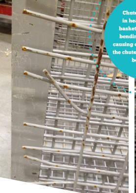
Chutes being stored in heavy-guage wire baskets. The wire was bending and breaking causing catch points where the chutes could potentially be damaged.
