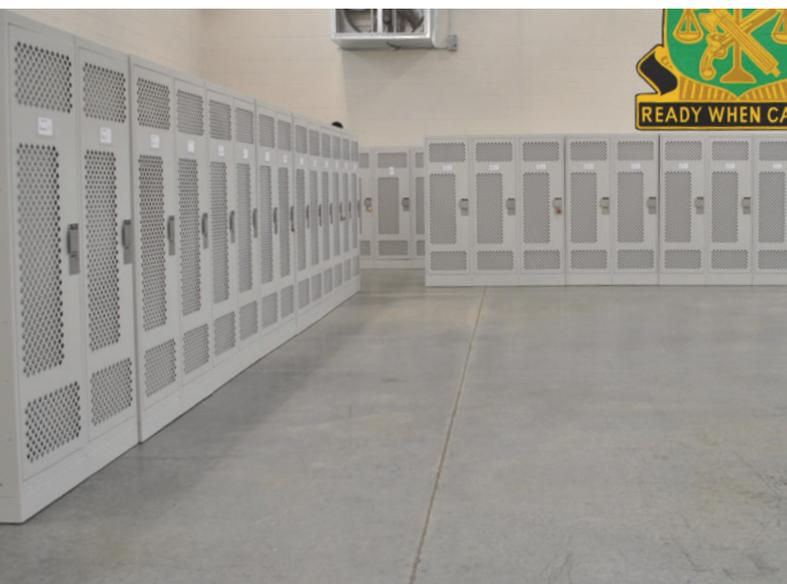
Each locker was constructed with a perforated mesh door designed to obscure the view of expensive equipment kept inside for added security.
