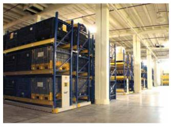
Spacesaver's **ActivRAC®** 16P System is designed for heavy applications, remote aisle activation, and all of the customizable and reconfigurable benefits of all of our systems. Multiple module systems can accomodate column considerations cost-effectively.
