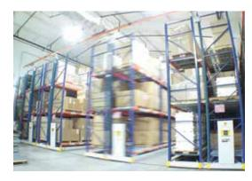
Installed on existing concrete slabs, our **ActivRAC** 16 Mobilized Storage System requires no costly structural footings or leveling. It's designed to articulate over reasonably unlevel flooring, while providing smooth operation.
