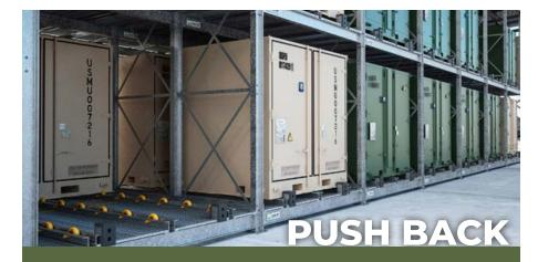
BAN-AIR PUSH BACK RACK is custom designed for dense storage where space is constrained, specifically to store both 463L & ISU90 containers. Heavy duty castors on each platform level allow the push back of ISU90/463L
