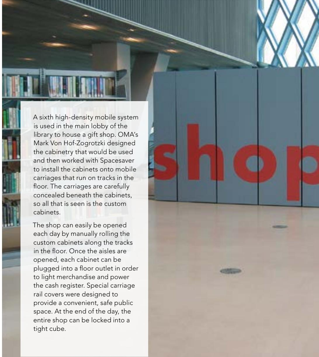
A sixth high-density mobile system is used in the main lobby of the library to house a gift shop. OMA's Mark Von Hof-Zogrotzki designed the cabinetry that would be used and then worked with Spacesaver to install the cabinets onto mobile carriages that run on tracks in the floor. The carriages are carefully concealed beneath the cabinets, so all that is seen is the custom cabinets.
