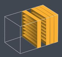
Mobile shelving optimizes storage more efficiently. Shelving units are placed on rails and aisles are opened at the point of need, allowing more items to be stored in LESS FLOOR SPACE.
