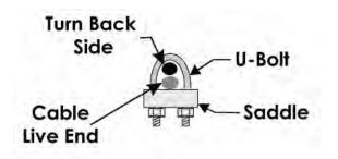
Tighten cable clamp hardware to 4.5 ft-lbs (6.1 N·m)
