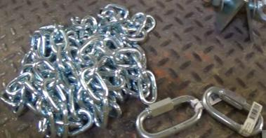
Z-Purlin ceilings require the GFY<sup>®</sup>Z-Purlin Kit for each of the (4) anchor points. Do NOT hang the TAZ fan from individual purlins.
