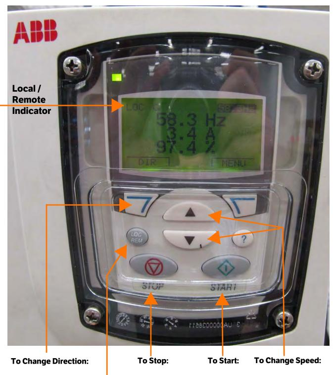
Local / Remote - Must be in "Local" for the controller to operate the fan. Look for "LOC" or "REM" if the upper left hand corner of the display.
