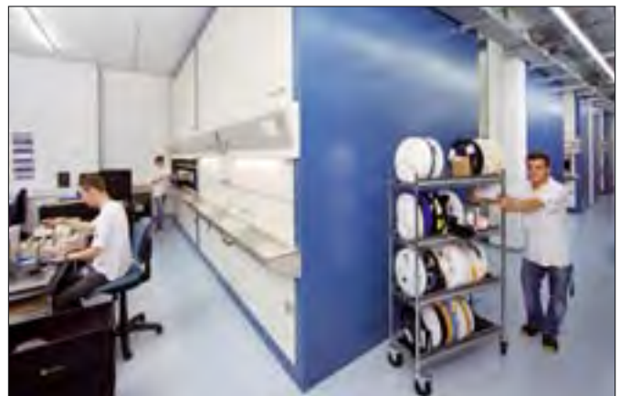
ESD buffer store for PC board assembly
