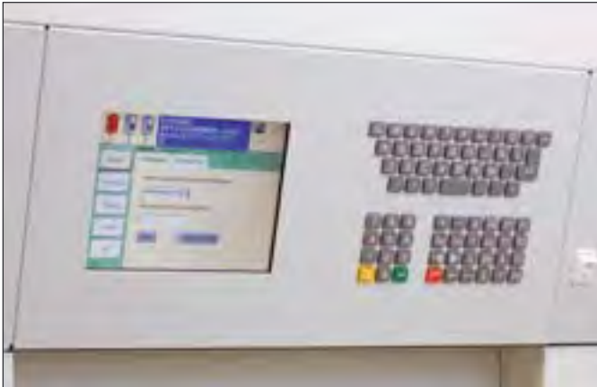
The Hänel MP 12 N-StandAlone top controller with touchscreen technology
